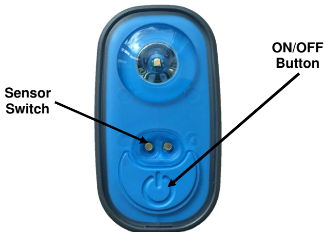
Figure depicts the Sensor Switch and the Manual ON/OFF Button
