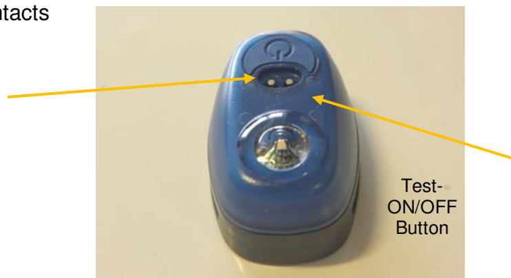
Figure depicts the Water activation contacts and the Manual Test Button.
