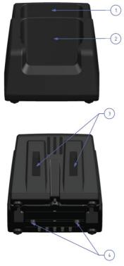
Figure 6: RH-30 Holder components
