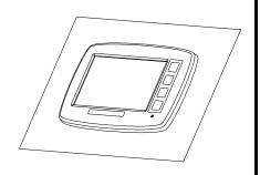
Install the sensor unit. The sensor unit on the mounting plate shall be installed on a horizontal surface and aligned with the ship's axis.
