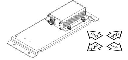
Accuracy of the sensor may be severely degraded due to misalignment during installation.
