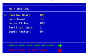
The desired menu option is chosen using the menu key. When the arrow cursor is alongside the appropriate option, pressing the up or down arrow keys changes the setting.
