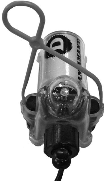
Although mounting methods will depend on the intended application, the single-pull toggle is intended to be attached to a suitable point on the liferaft such that it is dragged out of the battery unit when the liferaft is inflated, so illuminating both lamps. (For example, the battery unit may be attached to the roof of the liferaft, with the toggle being attached to a lower point by a lanyard.)
