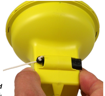
Release toggle attached, and switch moved to off position.
